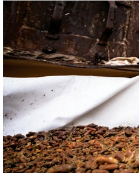
Working with local industries in al-Hasa, date palm waste is crushed into powder and added to drilling fluids to prevent the loss of circulation. This novel approach, under investigation by our R&D Center in Dhahran, could reduce costs and generate new business opportunities.
